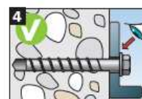
Once tightened, it must not be possible to turn the screw. The screw head must rest on the fixture and must not be damaged.
