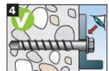
Once tightened, it must not be possible to turn the screw. The screw head must rest on the fixture and must not be damaged.
